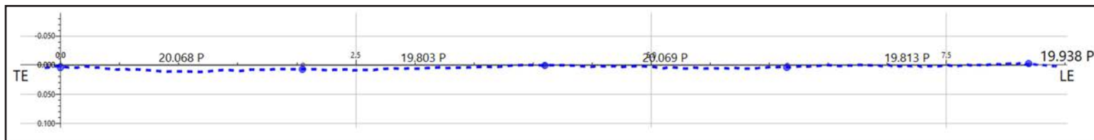
Figure 3- Flat-face/constant pitch 70R line with consistent local pitch values from TrueProp Software.
